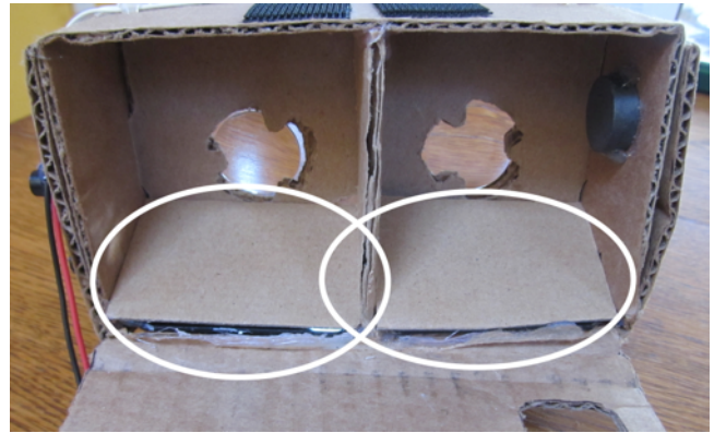
Figure 4: View Inside the Cardboard, with Baffles (circled in white) to Keep Light Out of the Viewing Chamber.
