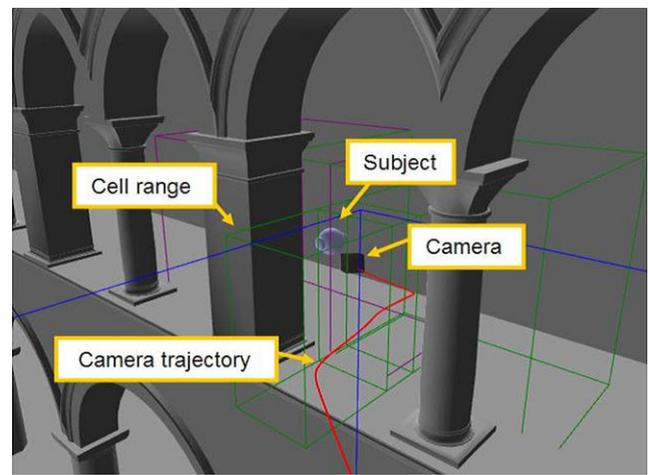
**Fig. 9** Camera trajectory near obstacles
