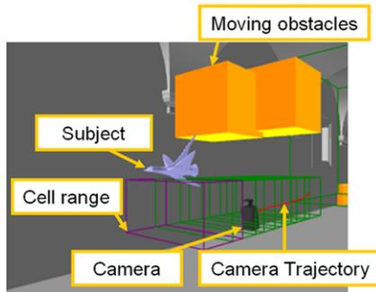
Fig. 11 Camera trajectory in dynamic environment
