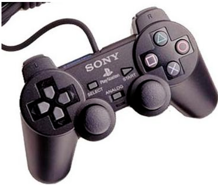
The Dual Shock 2. The analog sticks may be depressed, and most of the buttons are analog. ( amazon.com )
