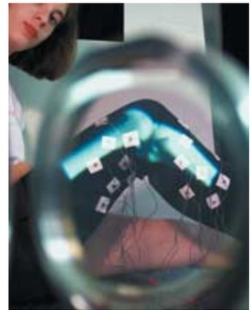
MEDICAL APPLICATION was built by researchers at the University of Central Florida. The system overlaid a model of a knee joint on the view of a woman’s leg. The researchers tracked the leg’s position using infrared LEDs. As the woman bent her knee, the graphics showed how the bones would move.
