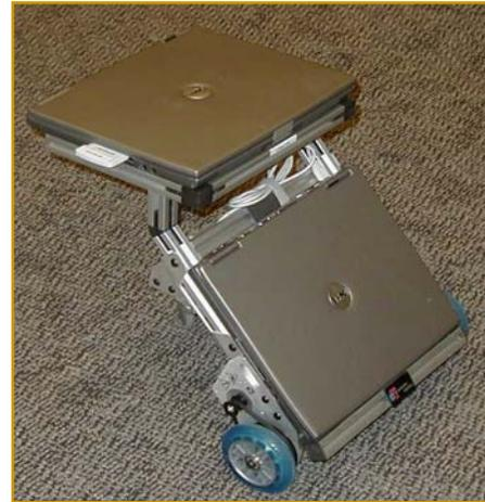
Figure 3 – Programmable robotic platform used in mobility tests
