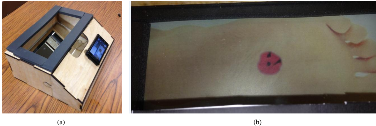
Figure 6. Design of image capture foot box. (a) photo of the actual foot box; note the smart phone; (b) sample image taken with the foot box.
