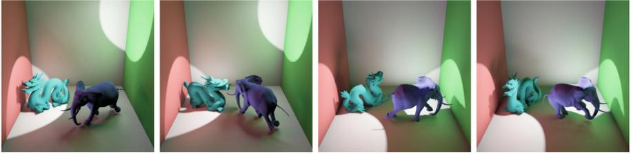
**Fig. 1.** Sample results using our technique: Dynamic Cornell box scene with dragon and running elephant rendered using two spot lights at 50 fps on an NVIDIA GeForce Titan X GPU. Indirect illumination is generated by 512 one-bounce virtual point lights
