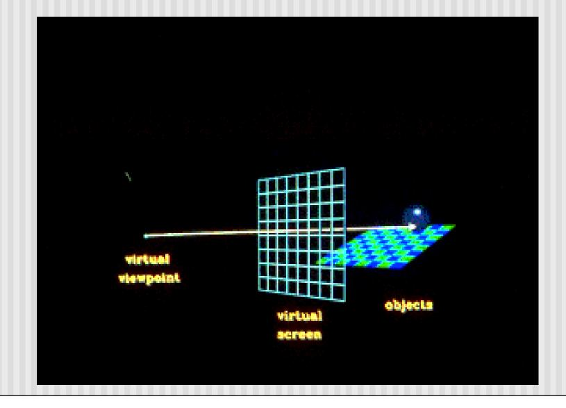
• Ray hits object: Check if hit point is in shadow, build secondary ray (shadow ray) towards light sources.
