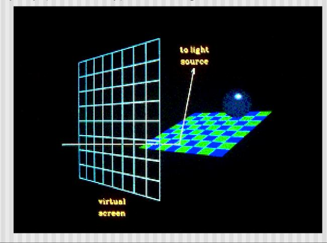
If shadow ray hits another object before light source: first intersection point is in shadow of the second object. Otherwise, collect light
