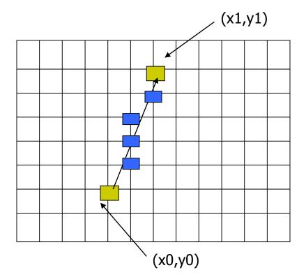
x = x0y = y0Illuminate pixel (round(x), y)y = y + 1x = x + 1/mIlluminate pixel (round(x), y)
