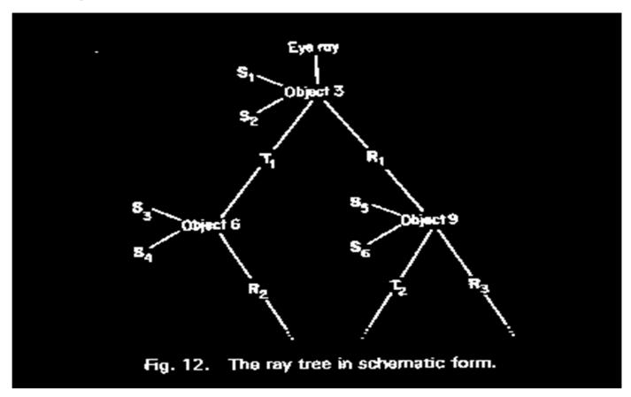
Reflective and/or transmitted rays are continually generated until ray leaves the scene without hitting any object or a preset recursion level has been reached.
