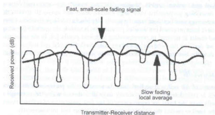
Figure 2.7 Variation of signal level according to transmitter-receiver distance
