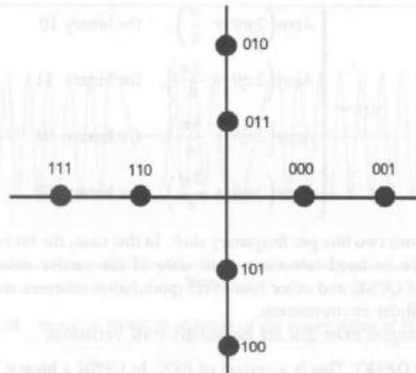
Figure 2.28 8-level QAM constellation encoding 3 bits/baud
