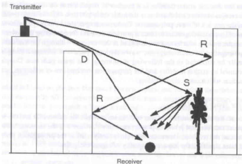
Figure 2.5 Reflection (R), diffraction (D) and scattering (S)
