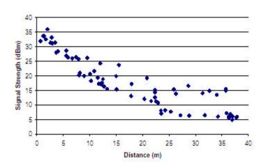
This other graph shows the signal strength as measured by intervening walls between the base station and the mobile host
