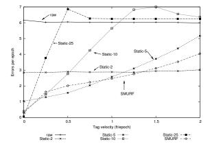
Figure 7: Average errors per epoch as tag velocities vary from 0 to 2 feet/epoch following *Pallet* behavior.
