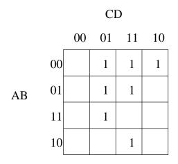
(a) (5 points) Write the sum-of-products equation from which this Karnaugh map is derived. (Don't provide a minimal function yet, just give the function that would lead to the Karnaugh map pictured above.)
