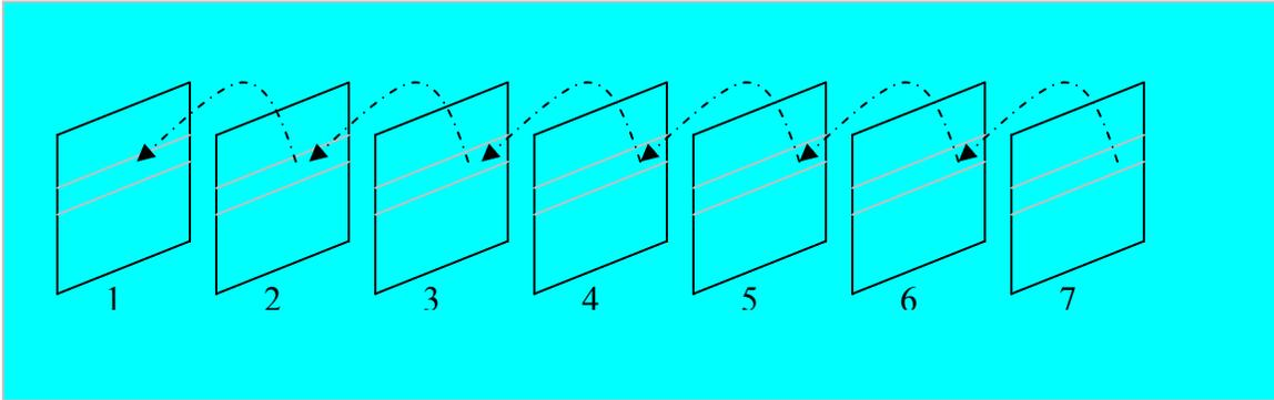
**Figure 4.0** Illustration of a reference chain, where each rectangle represents a video frame, the area between two lines in each rectangle represents a group of macroblocks (GOB), and the arrows indicate the selections of reference-GOB.
