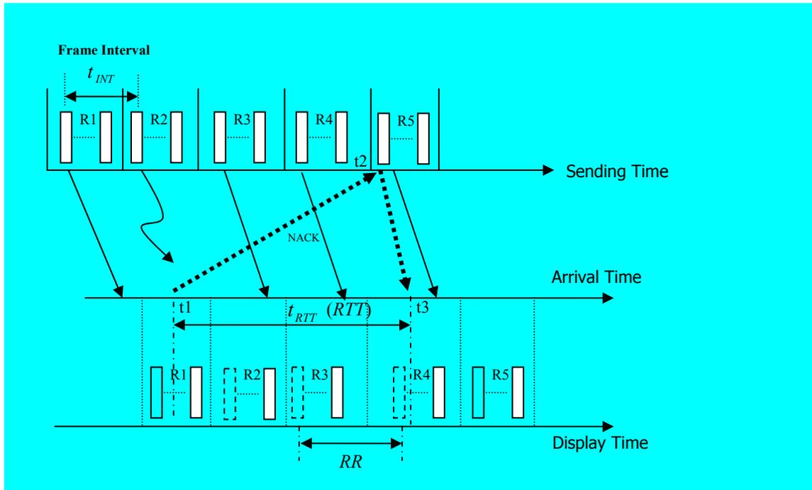
**Figure 4.1** Illustration of Retransmission Range (*RR*), where each rectangle represents a GOB, and the rectangle with dashed-line indicates the GOB is either lost or cannot be decoded correctly due to error propagation.
