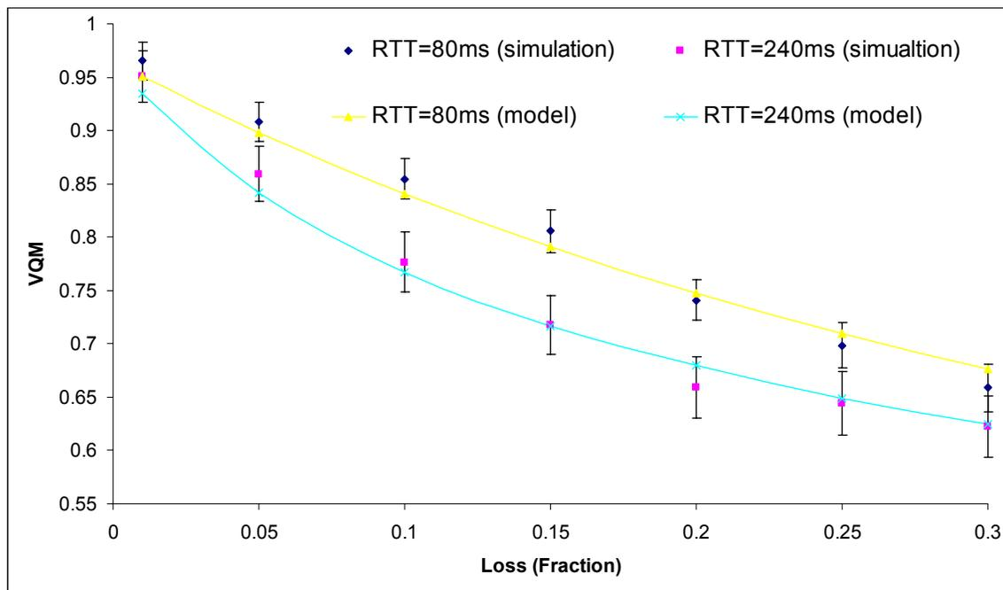
**Figure 6.10** VQM vs. loss with RPS NACK (video clip: Akiyo)
