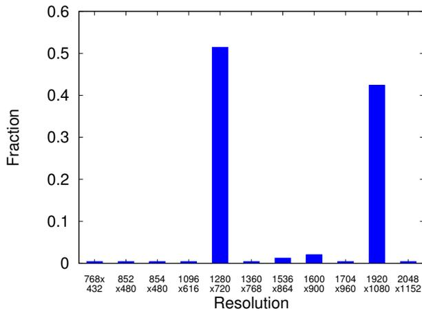
Fig. 3. Screen Resolutions. Histogram of live stream screen resolutions in pixels, ordered from lowest resolution to highest resolution.
