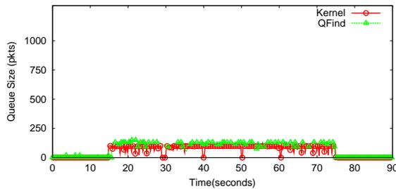
Fig. 6. Host AP with transmit queue length set to 100 packets.
