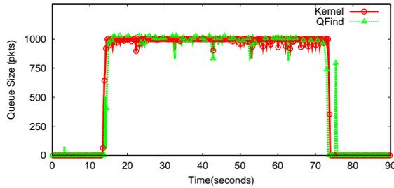
Fig. 5. Host AP with transmit queue length set to 1000 packets.
