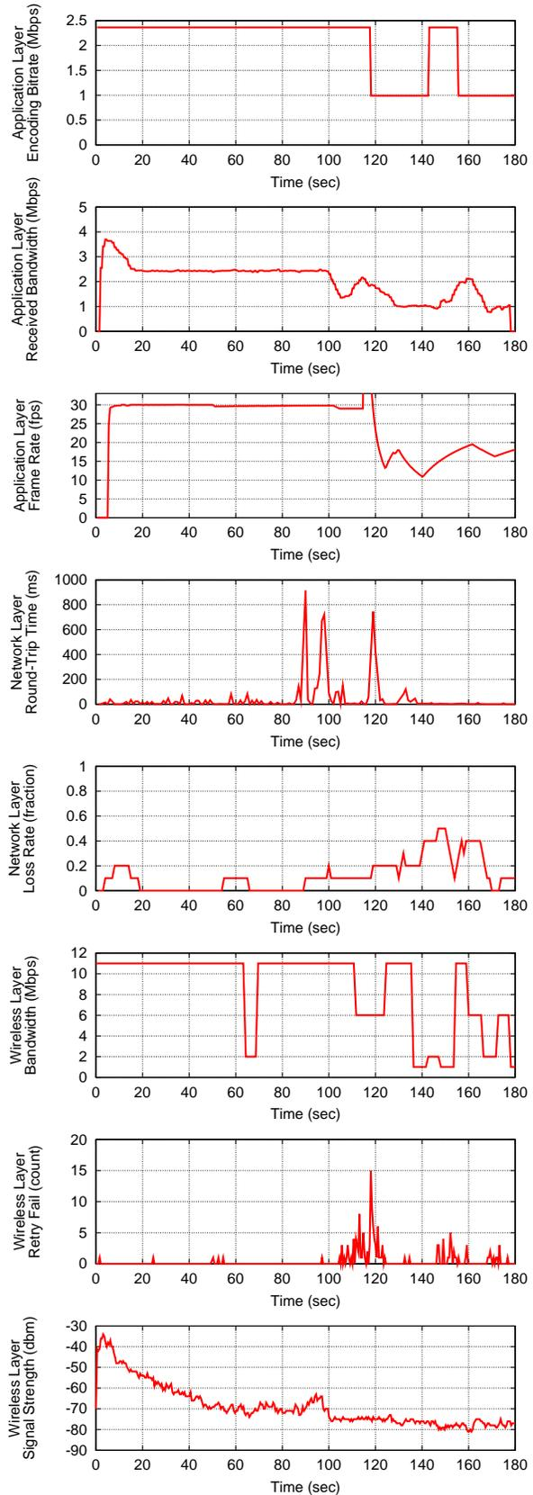
Fig. 2. Application layer, network layer, and wireless layer performance of a mobile client streaming a high-quality, multi-layer video clip.
