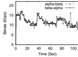
Figure 18: Bitrate versus Time with 1000 ms induced latency.
