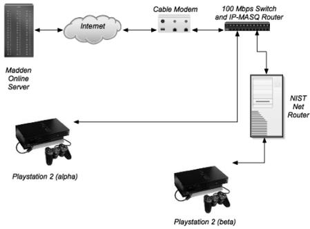
Figure 1: Experimental Testbed.
