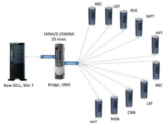
Fig. 2. Experiment setup
