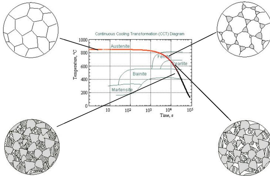
Fig. 7. CCT Diagram and Predicted Microstructures
