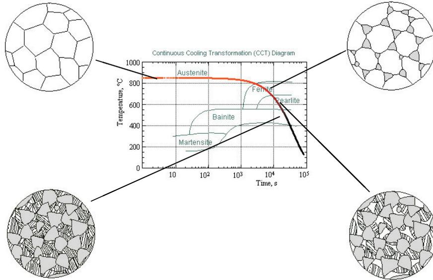
Fig. 7. CCT Diagram and Predicted Microstructures
