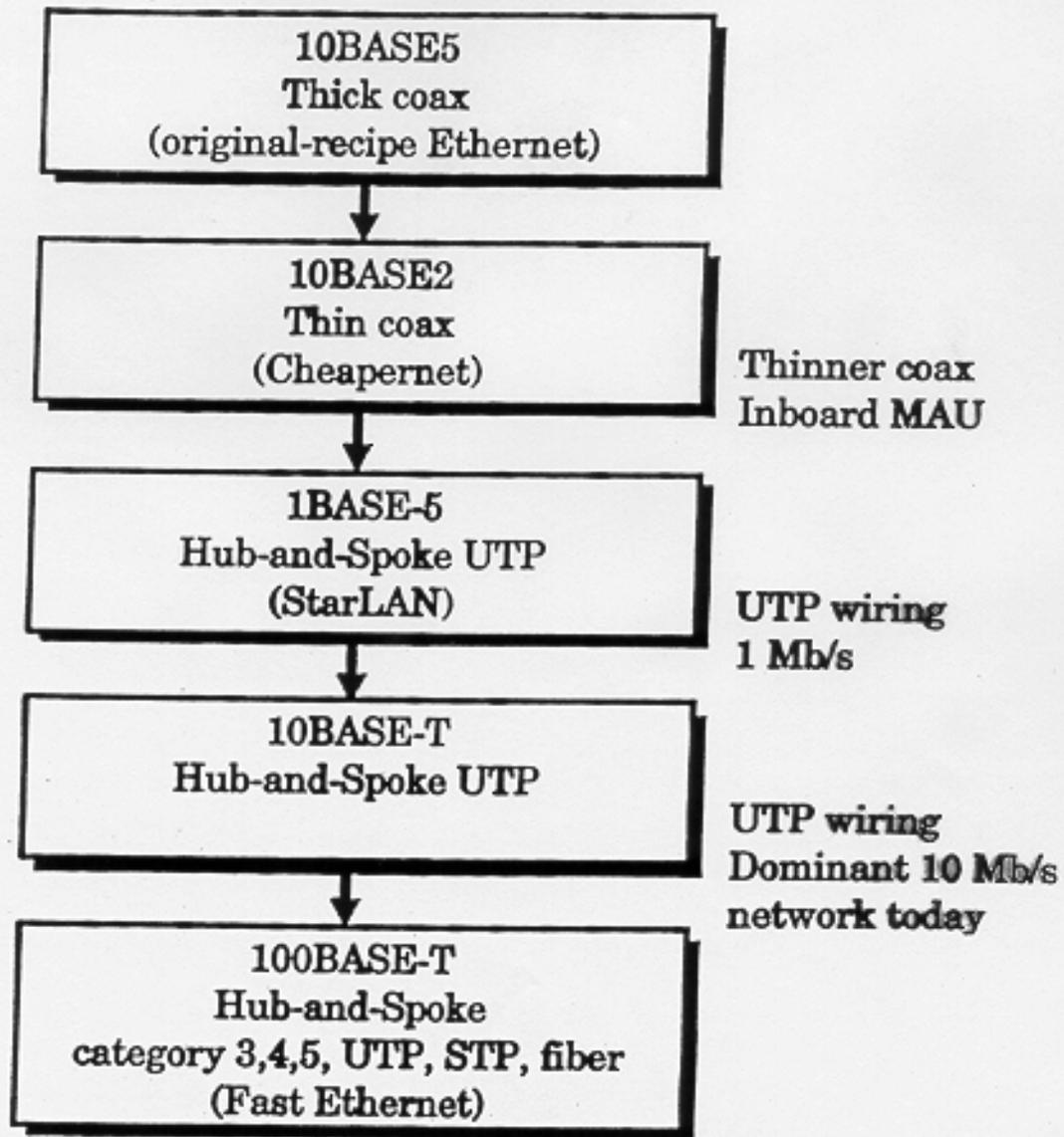
**Figure 1.4** Lineage of Fast Ethernet
