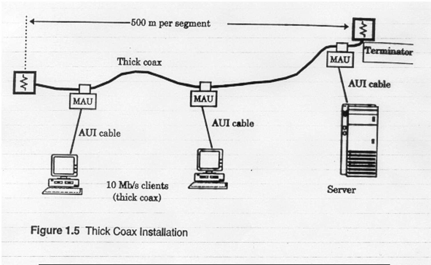
Figure 1.5 Thick Coax Installation
