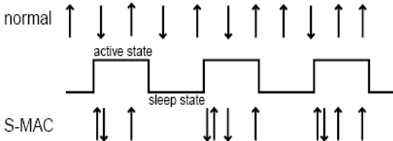
Figure 1: The S-MAC duty cycle; the arrows indicate transmitted and received messages; note that messages come closer together.
