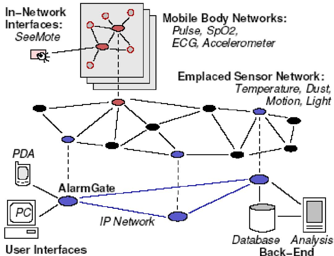
Figure 2. ALARM-NET architecture components and logical topology.
