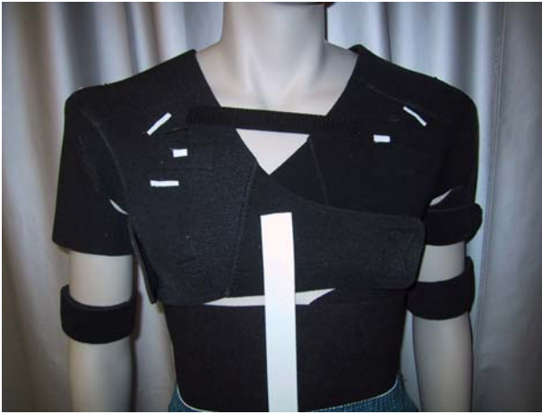
Fig. 7 The TactaVest (before wiring) is designed to hug the wearer through a large range of motion, while still granting adequate freedom of movement
