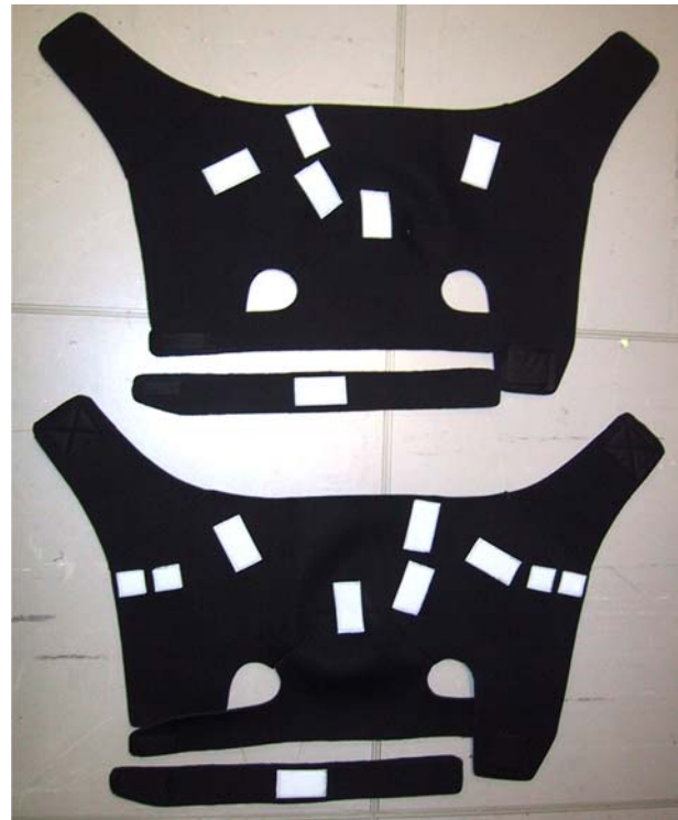
Fig. 8 The TactaVest is made up of five parts: two yoke-like shoulder pieces, two elbow bands, and a belt (not shown). The longer white hook-and-loop fastener pieces denote mounting points for the tactors
