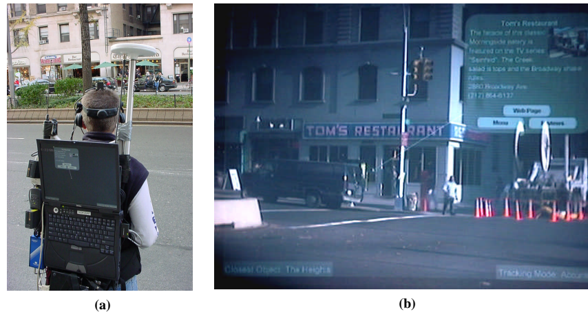
Figure 9.1 Mobile AR restaurant guide. (a) User with MARS backpack, looking at a restaurant. (b) Annotated view of restaurant, imaged through the head-worn display.
